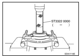
3. Using a drift (SST) and a puller (suitable tool), press wheel bearing outer side inner race out to remove from wheel hub.
