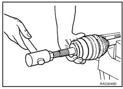
6. Install boot securely into grooves (indicated by \* marks) shown in the figure.
