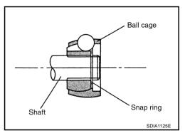
5. Apply the specified amount of grease (NISSAN genuine grease or equivalent) onto housing (\* point) and install it to shaft.
